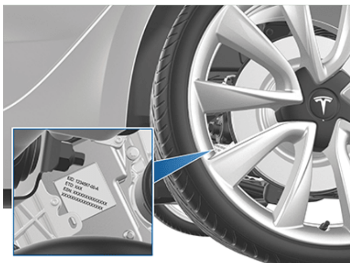
Rear motor label located on rear trunk:
