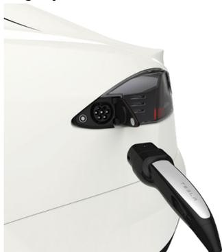
5. When you plug the Mobile Connector into your vehicle, a light beside the charge port pulses green during charging and the instrument panel displays charging information. The light turns off soon after the vehicle is locked.
