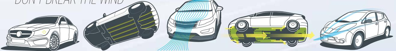
The Mercedes-Benz CLA250's aggressively beveled corners guide air around the side surfaces and into the wake with minimal disruption.
