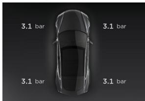
**Note:** If "Tire Pressure System Needs Service" displays after performing auto learning, try this procedure again. If the warning still persists after 5 minutes of driving at 40 km/h (25 mph), contact Tesla.
